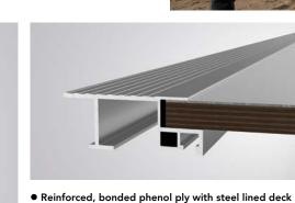
• Reinforced, bonded phenol ply with steel lined deck A brand new aluminium extrusion is a unique solution to the challenge of fixing the heavy duty deck into the chassis. Bonding the outer 2mm steel deck liner to the 18mm industrial grade phenol ply creates a very tough and durable load bearing surface, with the added benefit of easily discharging the load during tip operation.
