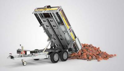
• Integral tie-down points inside the bed offer a significant benefit to any operator carrying machinery. Experience the convenience of multiple points, all as standard. Load loss is prevented with a spring steel flap.
