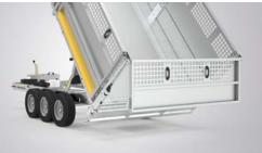
O High panelled side extension kits enable the transport of bulkier loads. Light weight, yet robust panels can be individually removed, along with the quick release retaining posts. This enhanced functionality makes Tipper2 easily configurable.
